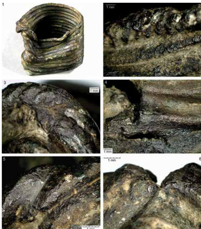
Fig. 10. Selected images from the macroscopic and microscopic observations: 1–6: multi-coil spiral bracelet no. 9; traces of impact (1), fractures of individual coils (4, 6), melting and fusion of some coils with each other (2–4), residues of charred organic matter (4)
